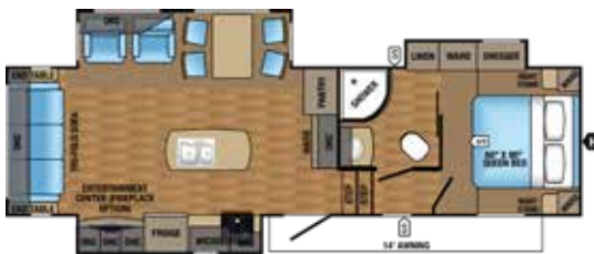
EAGLE HT FIFTH WHEEL | 28.5RSTS OPTION D Ext. Lgth: 32' 11" Ext. Ht: 142" Unloaded Wt (lbs.): 8,405 Sleeps: 3-4
