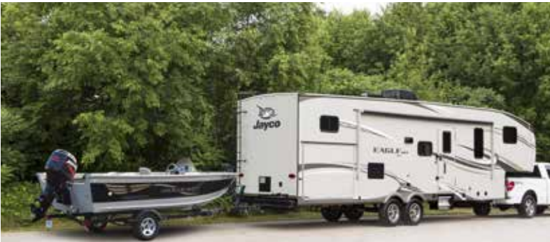
STANDARD INTEGRATED REAR 2-INCH RECEIVER HITCH WITH 300-POUND TONGUE CAPACITY AND 3,000-POUND TOW RATING (EAGLE HT ONLY)
